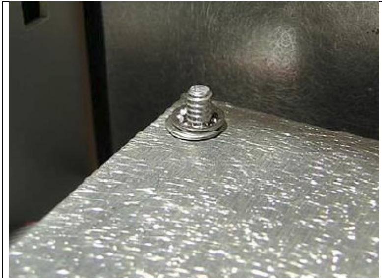
Figure 7 - Flat washer and internal tooth lock washers on top of RF shield
