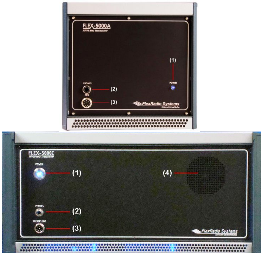
Figure 2: FLEX-5000A (top) and FLEX-5000C (bottom) Front Panel
