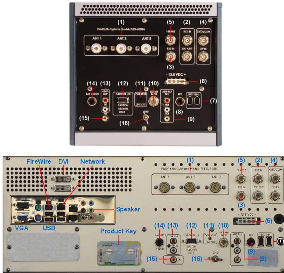
Figure 3: FLEX-5000A (top) and FLEX-5000C (bottom) Back Panel
