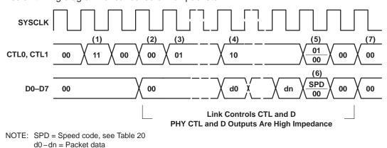
Figure 20. Normal Packet Transmission Timing
