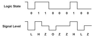
Figure 14. Signal Transformation for Digital Differentiation
