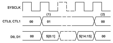
Figure 17. Status Transfer Timing
