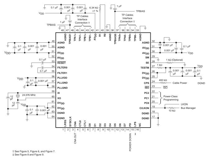
**Figure 4. External Component Connections**
