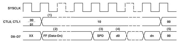
Figure 18. Normal Packet Reception Timing
