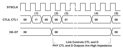
Figure 21. Cancelled/Null Packet Transmission
