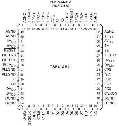
NOTE: Pin 16 (NC) could be tied to VDD for backward compatibility with the TSB41LV02A device.
