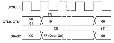
Figure 19. Null Packet Reception Timing
